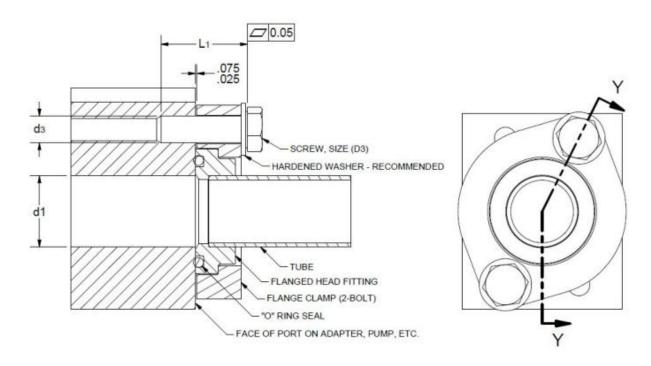
Dimensions, torques, and pressures for code 61 flange clamp assemblies type 1 with metric screw class 10.9.
